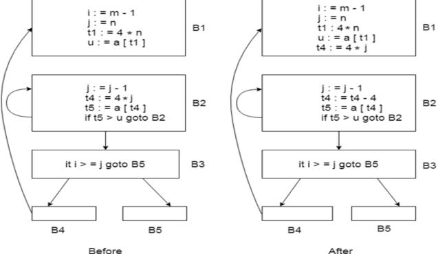
In this figure, we can replace the assignment t4:=4\*i by t4:=t4-4. The only problem which will be arose that t4 does not have a value when we enter block B2 for the first time. So we place a relation t4=4\*j on entry to the block B2.
